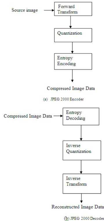
Fig 2. General block diagram of JPEG 2000
